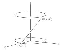
After rotation, that string joins (r, 0, 0) to (0, r, h') for some height h'. The midpoint of the segment is on the waist, at (r/2, r/2, h'/2), and the distance from this point to the central axis is  $\sqrt{(r/2)^2 + (r/2)^2} = r/\sqrt{2}$ .
